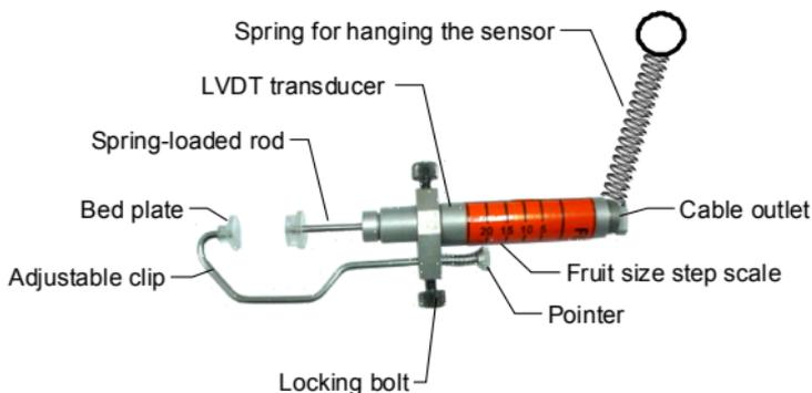
Standard cable length between sensor and signal conditioner is 1 meter. The output cable length should be specified in the order if required.
