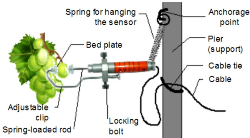
A stationary pier (support) is to be used for positioning the sensor and its cable. At first, adjust the sensor's clip to the fruit diameter by using a step scale located on the sensor's body.
