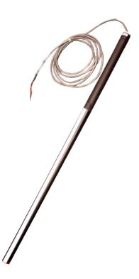
An alternate method of packing the soil against the sensor is to prepare slurry from the native soil and fill the hole. Then insert the sensor. The slurry will help fill the space between the sensor and the soil. Horizontal sensors would be installed in a trench and then back filled and packed. For further information log onto our web site, click on "products" and scroll down to the "instruction manual for TDR." CAUTION: DO NOT leave sensor lying out in the direct sun prior to installation.
